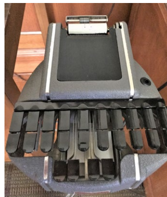
Today's Stenotype machines look much like this vintage one—24 unmarked keys. The letters the reporter writes today go into a computer instead of onto a narrow roll of paper, as shown here. Reporters “do not say ‘type’ in the industry; we say ‘write,’” Lockwood said.
